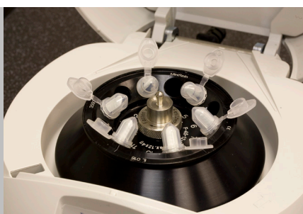
Spin + Collect Sample Recovery Device requires a single centrifugation step
